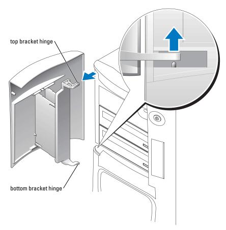
**3** Lift the bottom bracket hinge away from the computer.
