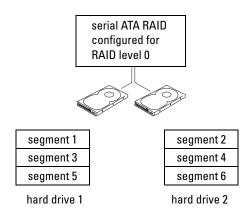
Another advantage of a RAID level 0 configuration is that it utilizes the full capacities of the drives. For example, if you have two 120-GB drives installed, you have 240 GB on which to store data.
