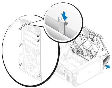
4 Close the computer cover halfway and pull the front panel away from the computer.
