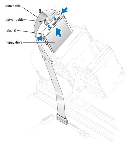
**4** Press inward on the two tabs on the sides of the drive, slide the drive upward, and remove it from the floppy-drive bay.
