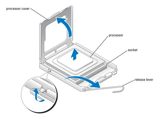
Remove the processor from the socket. Leave the release lever extended in the release position so that the socket is ready for the new processor.
