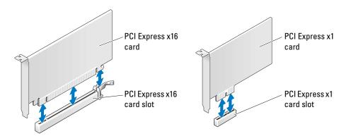
If you are installing or replacing a PCI Express card, follow the procedures in the next section. If you are removing but not replacing a PCI Express card, see "Removing a PCI Express Card" on page 89.
