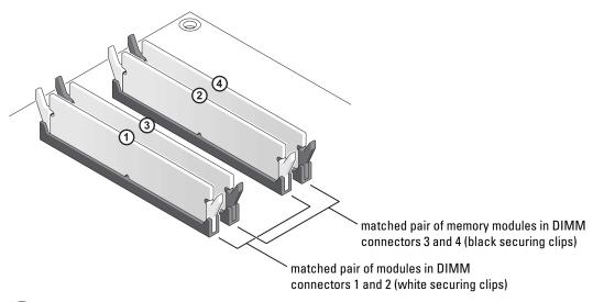
**NOTICE:** If you remove your original memory modules from the computer during a memory upgrade, keep them separate from any new modules that you may have, even if you purchased the new modules from Dell. If possible, do not pair an original memory module with a new memory module. Otherwise, your computer may not start properly. You should install your original memory modules in pairs either in DIMM connectors 1 and 2 or DIMM connectors 3 and 4.
