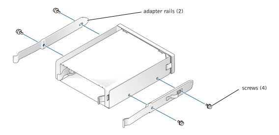
6 Slide the adapter into the 5.25-inch drive bay until the tabs on the rails securely click into position.
