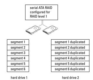
If a drive failure occurs, subsequent read and write operations are directed to the surviving drive. A replacement drive can then be rebuilt using the data from the surviving drive. Also, because data is duplicated on both drives, a RAID level 1 configuration using two 120-GB hard drives collectively has a maximum of 120 GB on which to store data.
